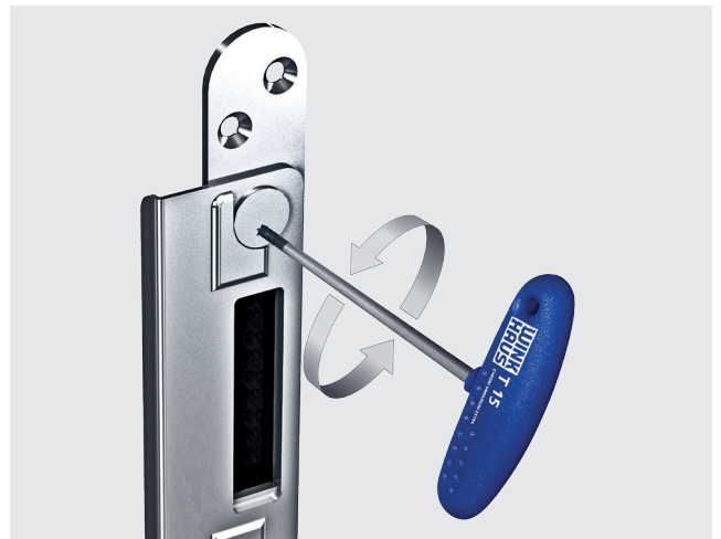
Keeps fully adjustable \pm 2 mm utilising Torx T15 adjusting tool.
