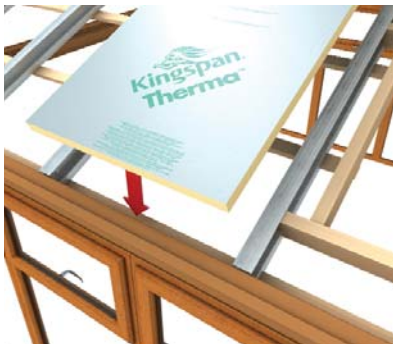
Install external insulation
