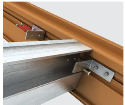
Fix rafters to ringbeam
